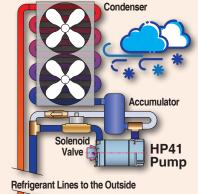
When the outside temperatures become low enough to maintain the desired cooling temperature, there is no need to compress the refrigerant to a higher pressure/temperature.
